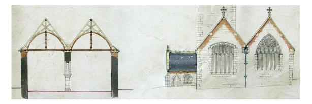
The two separate roofs were rebuilt in the 1870s restoration and are now of equal height, as per J P Seddon's plan above. Any original timbers seem to have been lost.
